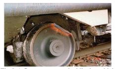
Fig 5. A flat spot occurred while the vehicle wheel set is dragging along the rail
